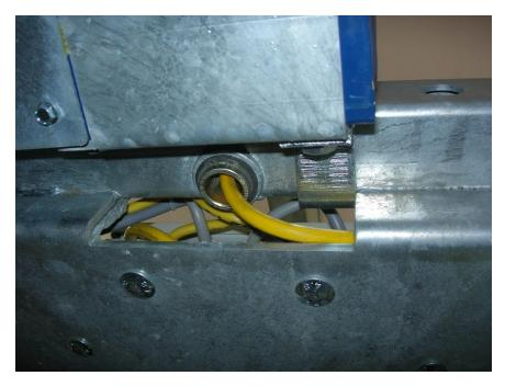
Insert the service arm and cable feed together with the tube into the bush and secure with the retaining ring.
