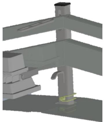
Place the service arm stop onto the molded tube as shown above and lock the locking pin into position – use elastic band for securing the service arm cable feed.
